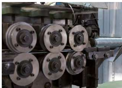
Profilatrice tubo flessibile Flexible conduit forming machine
